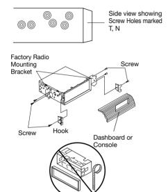
To fasten the unit to the factory radio mounting brackets.
